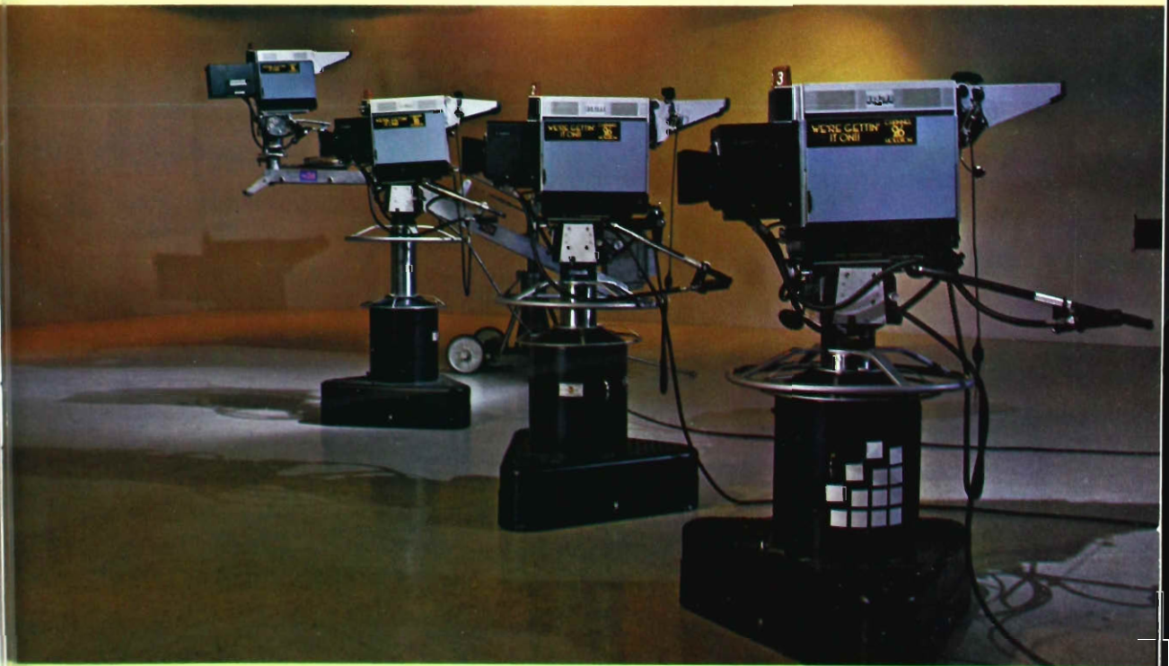
Battery of TK-44 studio cameras gives TV-26 superior color capability for commercials and local programming. Normal studio complement is three TK-44's, with two additional units available from the mobile truck.
