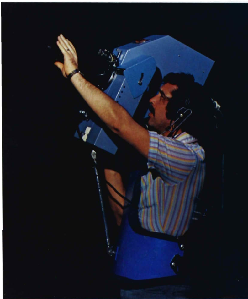
Telescoping camera support rod and hinged shoulder mount make it easy to tilt camera for angle shots.
