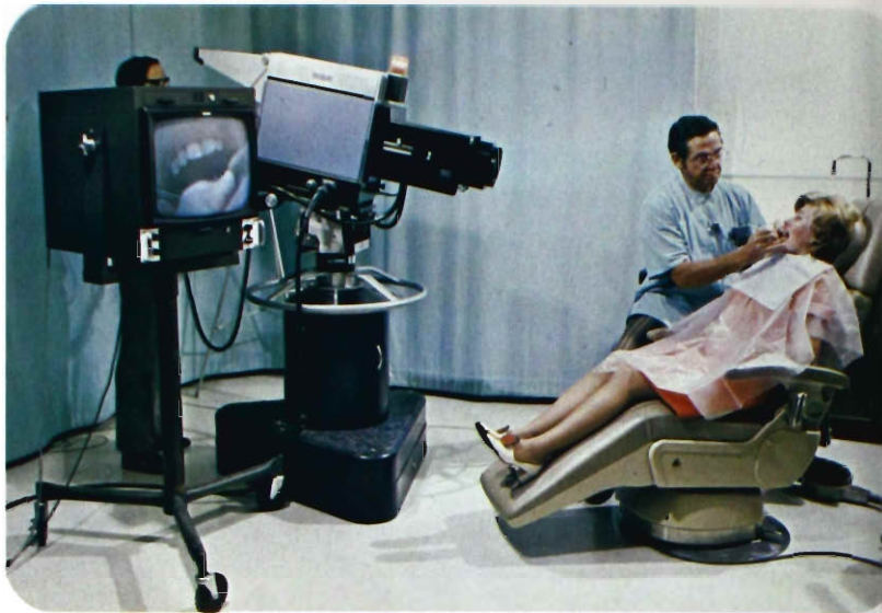
In recording Periodontal Procedures a second TK-44 is used for tight intra-oral closeups.
