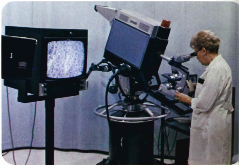
Instructor in Oral Pathology uses TK-44 with special microscope mount to show slide to Dental Hygiene students viewing in one of the school's main lecture rooms. The microscope mount was designed by Chief Engineer Ike Church.
