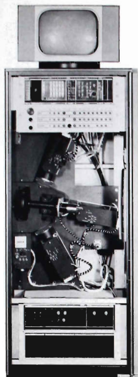
10. Single cabinet color film camera configuration.
