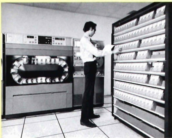
Instant access to current "card" commercials is provided by mobile storage rack designed by KVRL.
